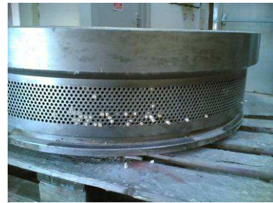
Pellet die producing 6mm pellets
