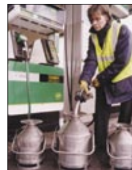
Inspection: A Trading Standards Officer checks the accuracy of a petrol pump.
